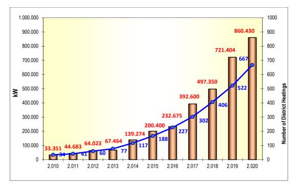
Figure 37: Evolution of the number of district heatings in Spain and its power. Predictions from 2016 to 2020. Source: AVEBIOM
