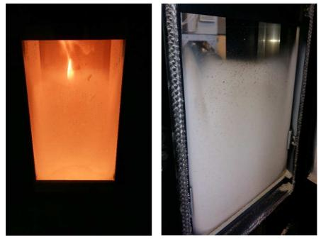
Figure 3.2. Severe aerosol depositions contamination of the vision panel during operation with OTP and VYP observed at Stove III
