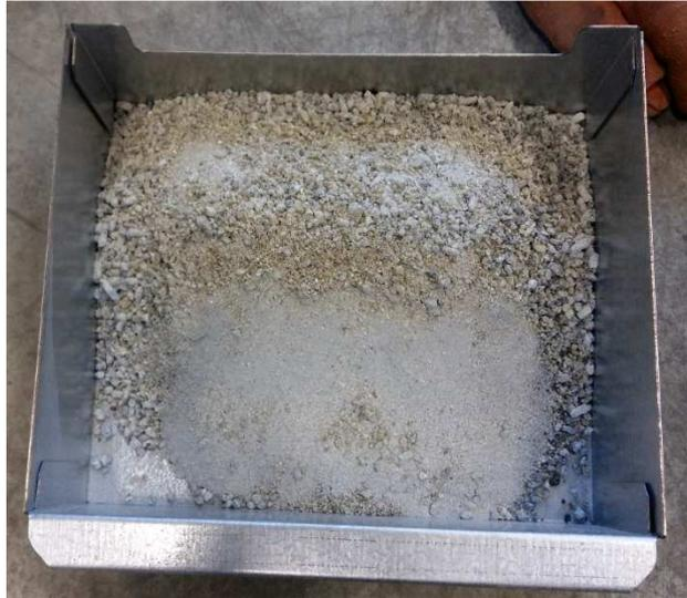
*Figure 3.1. Ash box of Stove III after test runs with OTP - OTP and VYP keep their shape during combustion due to their high ash contents*
