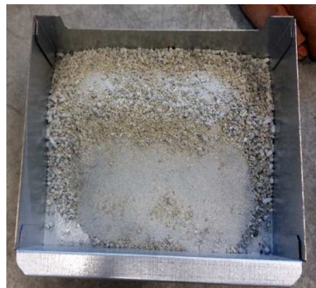
Figure 3: Ash box of Stove/BIOS after test runs with OTP - OTP and VYP pellets keep their shape during combustion due to their high ash contents
